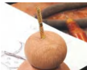
▲ Pic.11 Drill a hole at an angle in the head, use a double-ended screw and attach using a little PVA glue
